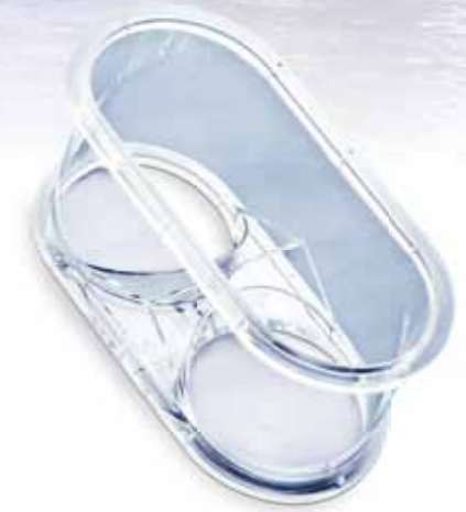
Custom PLEXIGLAS® double hopper with the tightest tolerance specifications, with hand formed and bonded sidewalls and CNC processed bonded flanges. Dimensions approx. 700 x 280 x 300 mm.
